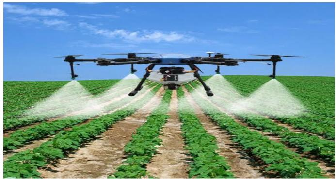
The device is far superior to manual spraying because it is much faster and ensures uniform pesticide spraying across the entire crop. As drones do not contact the soil, they can help to avoid crop damage caused by compaction.
